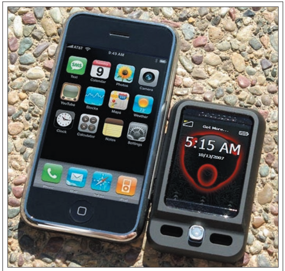
Fig. 2: The Apple iPhone with projected-capacitive touch (left) and the Neonode N2 cell phone with traditional optical touch (right). Photo courtesy of PenComputing.com.
