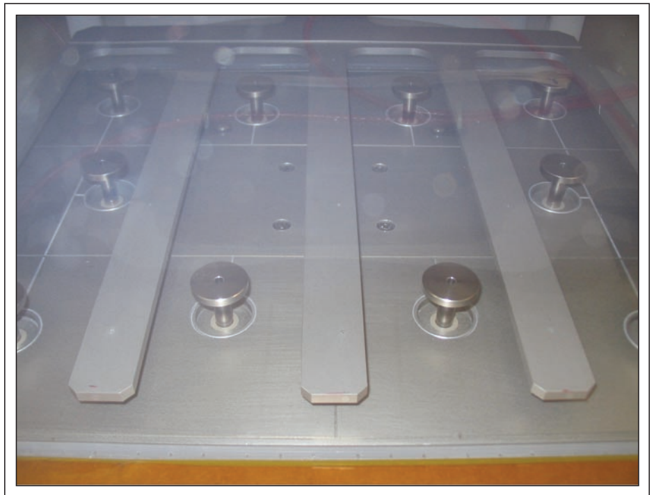
Fig. 5: Above is an example of a flexible-substrate transfer paddle and spin chuck with integrated lift pads
